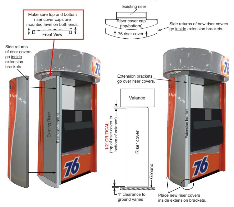
Place riser cover <u>between</u> extension brackets (<u>extension brackets overlap sides of riser cover</u>). Attach by driving K-lathe screws (painted to match extension brackets) thru extension brackets into sides of riser cover. Top and bottom K-lathe screws pass thru side tabs of top and bottom riser cover caps. Install two riser covers per dispenser.
