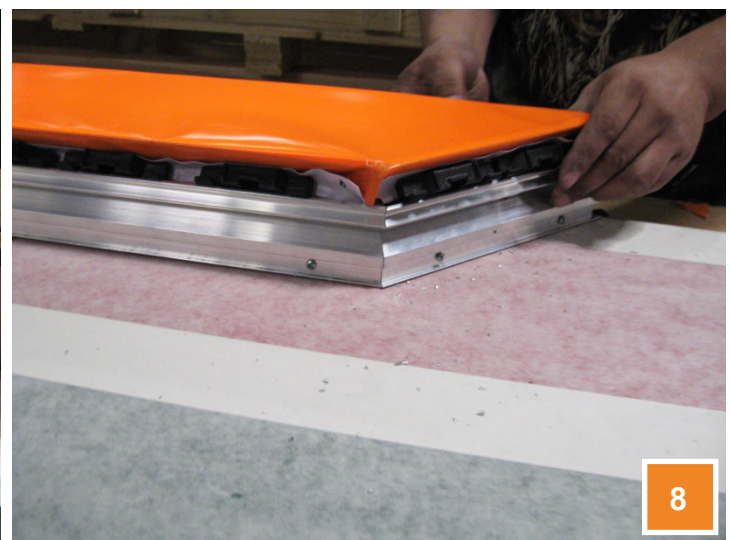
(Above) Continue moving along the face, repeating the above steps until reaching the end. If there is additional face after all tightening has been completed, clip the face carefully to trim it up.
